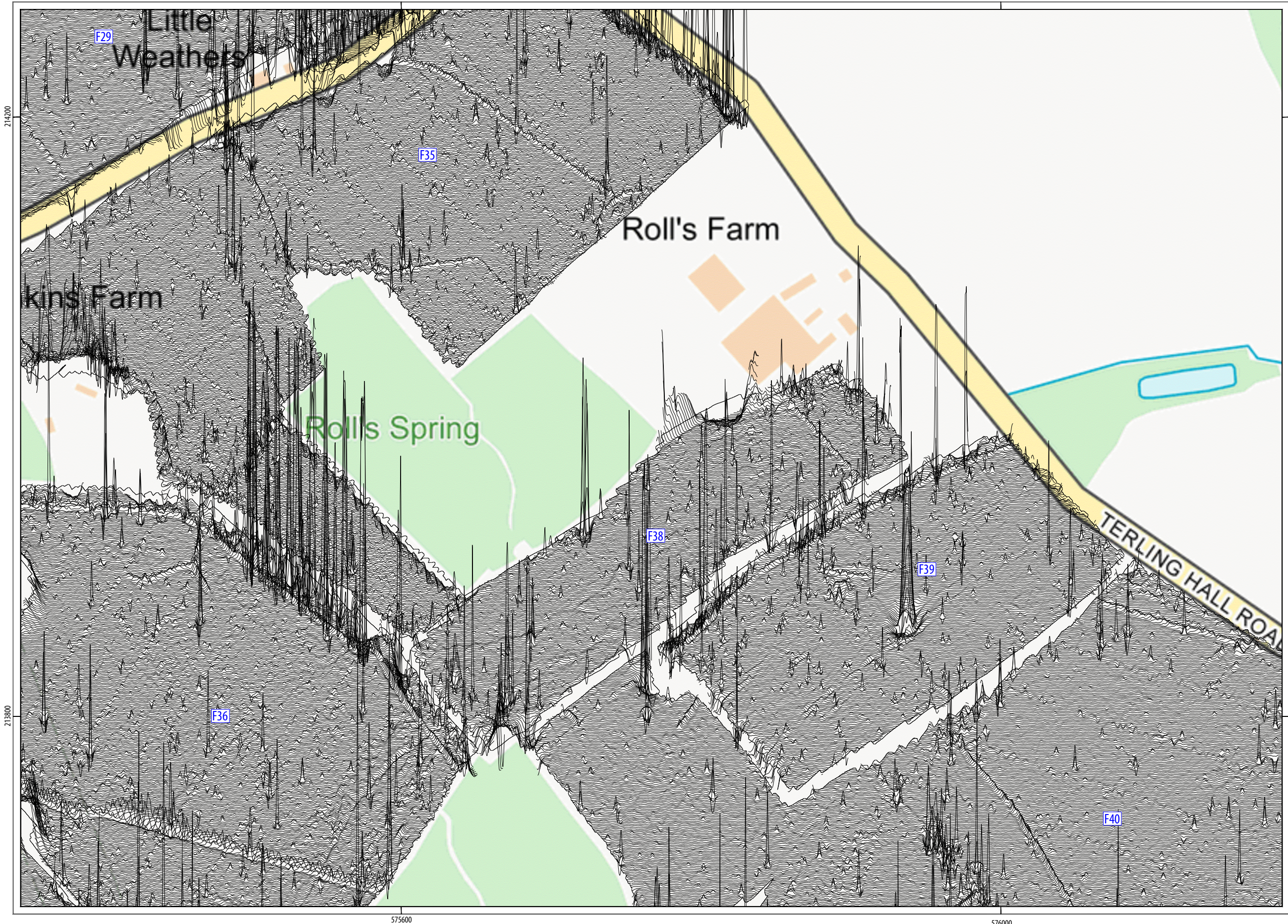
ILLUS 44 XY trace plot of minimally processed magnetometer data; Area 11
